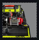
A front winch can be also equipped, providing enhanced capability for pulling, lifting, or recovering materials in demanding operations.
