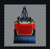
Used to move away and drag the remains of combustible materials produced by the chopper, as well as rocks and thick fuels.
