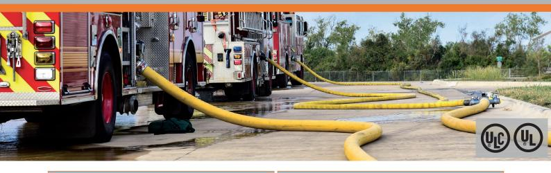
Superior nitrile/PVC rubber hose for use in supply and attack operations
