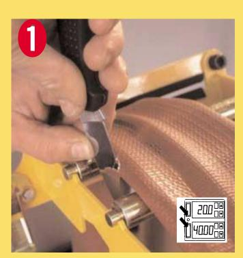
For best results dry the hose internally and externally. Switch Stenor Merlin to "On" and "Constant" to heat up. This will take around 8 minutes, and will heat whilst you carry out the preparation. Mount the hose clamp in a vice as shown here, with the round bars in place. Fold the hose in the clamp with the injured area closest to you. Cut a round hole about 8mm in diameter around the injury. This hole may be bigger than
