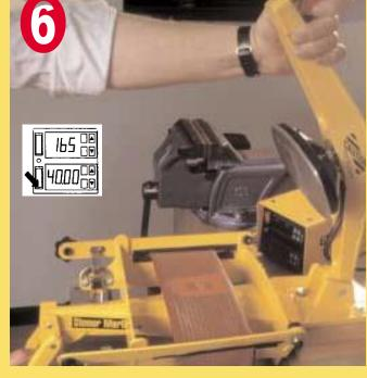
Make sure the vulcaniser has reached 165°C. Bring the top arm over and use the overcentre lever to apply the pressure. Switch to "Timed" and the timer will start to count down. The units on the timer are minutes and
