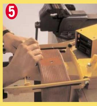
Check the plug patch position. When you are satisfied with its position, remove the nylon and discard it. Cover with a piece of cellophane to stop the patch sticking to the heating unit.
