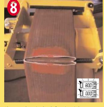
Alarm sounds to signal end of repair, switch to "Constant" to reset timer and switch "Off". If you are new to this technique of hose repair, then try it out on some condemned hose and cut the hose open.
