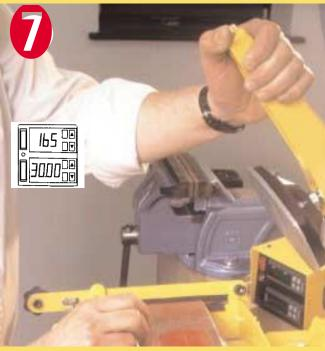
When the timer shows 30.00 (after 10 min) release the top arm and remove the cellophane. Having removed the polythene from the underside of the external patch apply the patch. The arrows are on the top.
