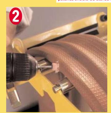
Mount the stone in a drill and prepare the inside of the hose carefully. A drill speed of less than 1200 rpm is recommended to avoid excessive damage to the internal hose wall. If you are new to this method, practice on some condemned hose a few times and cut the hose open and inspect the preparation. This will help you to get "a feel" for the internal preparation.
