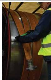
Hoses are tested in accordance with BS6391:2009 which stipulates an annual test pressure of 1.5 x maximum working pressure. Dependent on the customer's requirements we hydrostatically test hoses at between 12 and 22.5 bar (174 - 326 p.s.i.) Hoses that fail the test have areas of damage marked for repair, unique asset marks/numbers are recorded and logged on a spreadsheet and the failed hoses are set to one side.
