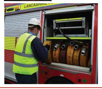
Once all testing is completed, a certificate is issued detailing the unique identifiers of the hoses that passed. The asset no./identifier acts as the key to all the other information recorded about the hose such as hose type, length, diameter, coupling make and age, test dates and history, giving a complete and comprehensive set of records in the event of an incident or accident. This record is also very useful when budgeting for replacement hoses.
