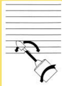
Move the hose in the clamp, so the injury is uppermost, and carry out the external preparation with the wire brush and drill. Prepare an area greater than the size of the patch to allow for the patch spreading. Avoid excessive material removal and damage to the fabric.
